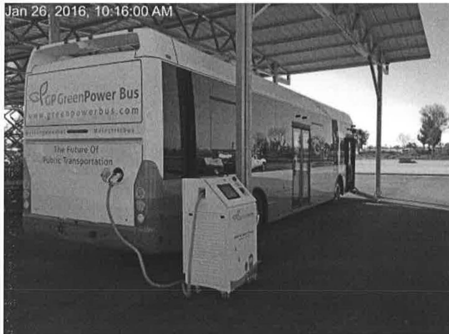
Figure 2 – GreenPower bus and mobile charging station under bus canopy
