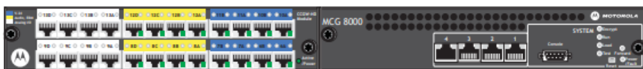
Figure 1-2: Enhanced MCG 8000 Conventional Channel Gateway—Connects dispatch operators to analog or digital conventional channels in the system
